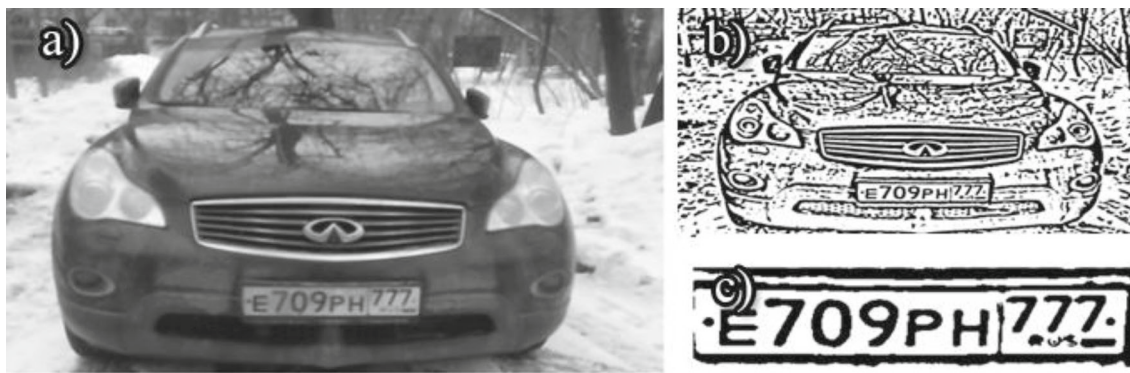
Fig. 3 Results of applying the Viola-Jones method for license plate recognition a converting the original image to grayscale using a Gaussian filter, b adaptive image binarization, c detected license plate
