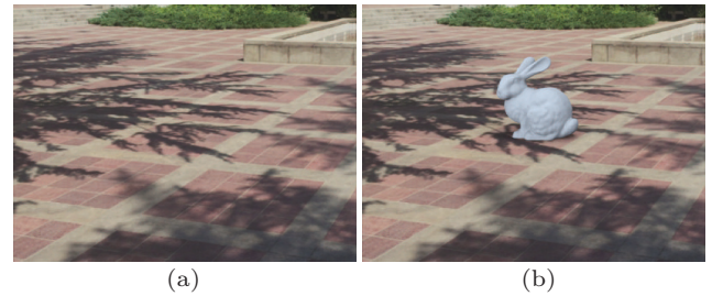
Fig.13. Our method cannot model complex illumination which cannot be represented by an environment map, e.g., shadows cast by objects outside the video frame. (a) Hard shadows are cast by a tree outside the frame. (b) Our method fails to recover the illumination, so hard shadows are not produced on the bunny added to the scene.
