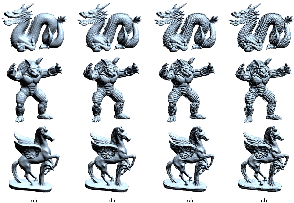
Fig.5. Relief detail exaggeration results for Dragon, Armadillo and Pegaso model using different manipulation parameters. (a) Original models. Different detail exaggeration results using two manipulation parameters (a, b) : (b) (1.0, 2.0). (c) (3.0, 2.0). (d) (3.0, 4.0).
