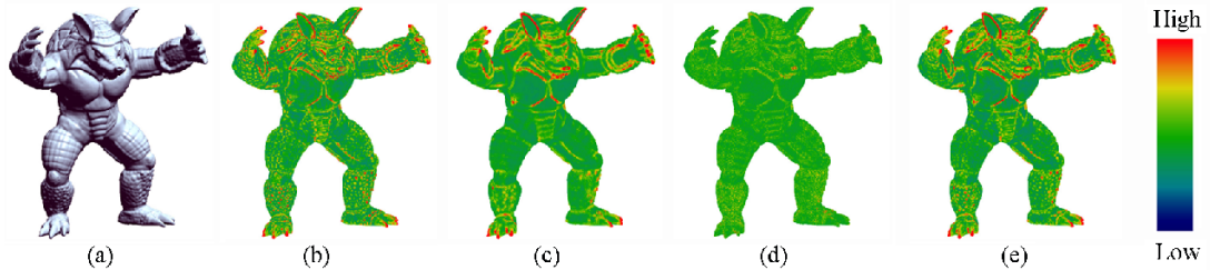
Fig.1. Multi-channel saliency computation steps for Armadillo model. (a) Original Armadillo model. (b), (c), (d) Feature maps of local height distribution, normal difference, and mean curvature variation, respectively. (e) Final combined multi-channel saliency map.
