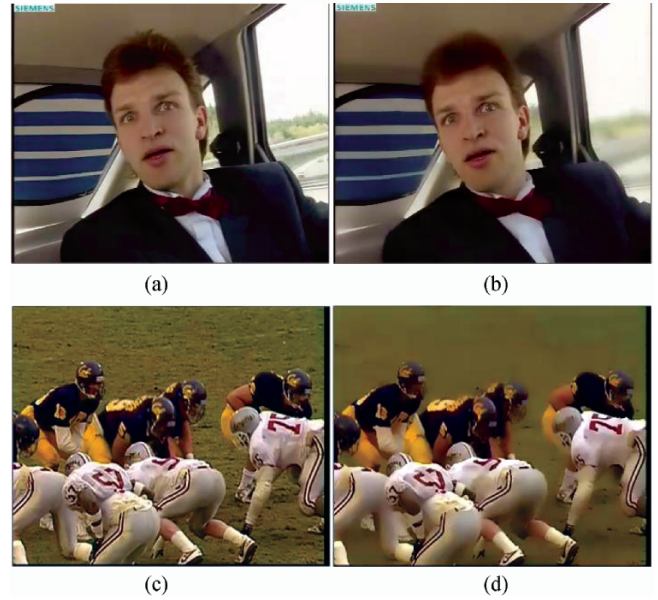
Fig.6. Comparison of results with QP = 28 . Note that in our result the face and the player's bodies are well preserved while uniform areas are smoothed. (a) JM12.0 result (292 kbps). (b) Our result (243 kbps). (c) JM12.0 result (1843 kbps). (d) our result (1120 kbps).
