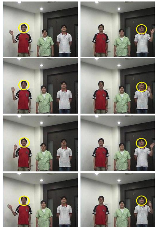
Fig.6. Sustaining and shifting attention guided by a motion cue. The task for the model is to find the person who is waving his hand. The model's attention is focused on the face of the person waving his hand as shown in each column, and when that person stops waving his hand and a second person starts, the model again shifts its focus to the second person's face.
