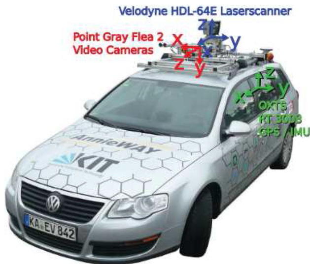
Fig. 10 The sensor suite platform of KITTI. The KITTI datasets are recorded on a passenger vehicle which is equipped with a pair of color cameras, two greyscale cameras, a Velodyne HDL-64E laser scanner and an OXTS GPS/IMU inertial navigation system which is used for providing ground-truth poses. This picture is taken from http://www.cvlibs.net/datasets/kitti/
