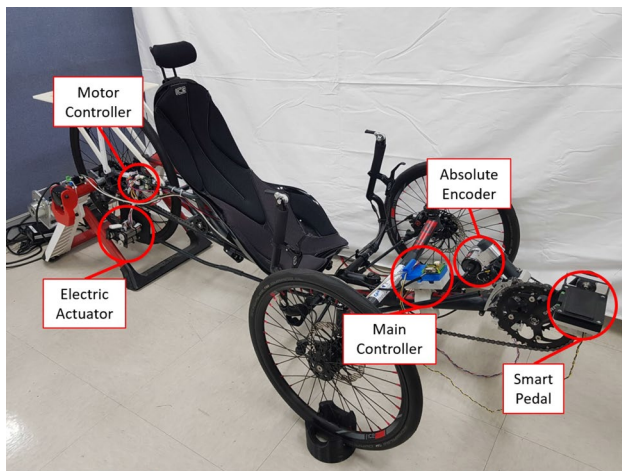
Fig. 2 Power-assisted trike developed in this study
