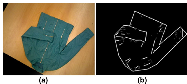
Fig. 6 Extraction of edges on the surface of a garment: a the colour image of the garment, b the extracted edges using depth information (colour figure online)
