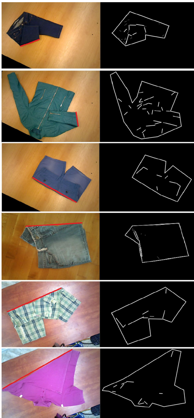
Fig. 21 Results of successful axis detection method in various garments. The colour image with the axis marked in red and the extracted edges from the depth image are provided for each example (colour figure online)
