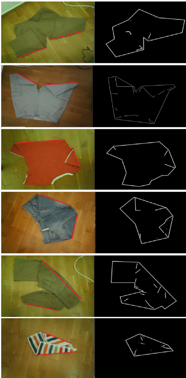
Fig. 23 Results of successful axis detection in cases with two folds. The colour image with the axis marked in red and the extracted edges from the depth image are provided for each example (colour figure online)
