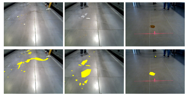
Fig. 12 Some frames taken from our dirt dataset. The top row shows the raw frames, and the bottom row shows the masked dirt in yellow. The two columns on the left depict frames captured in a supermarket, while the rightmost column is captured during a mission in an open space in an airport. During this mission, the proactive safety module was active. Since its red laser markings would interfere with dirt detection, it is masked out in that processing step. The dataset provides masks for dirt, floor, and said laser markings
