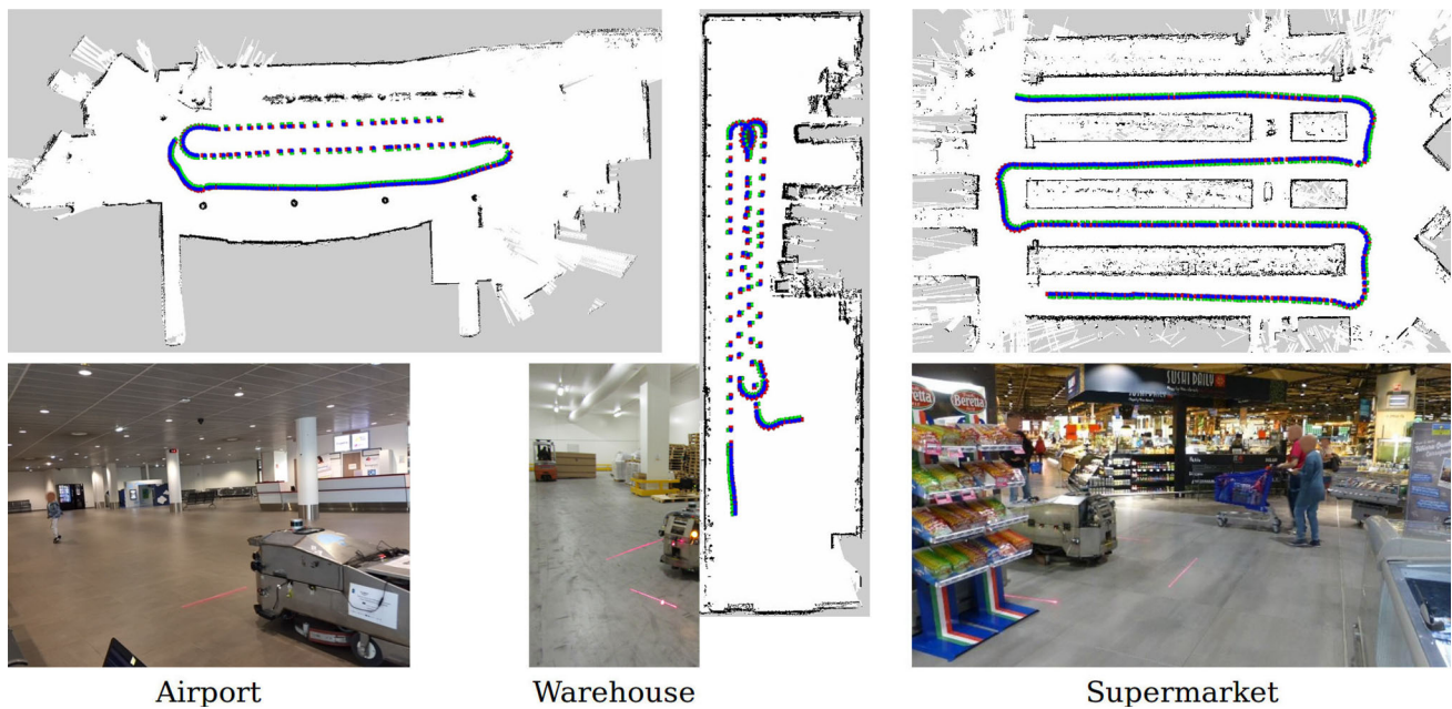
Fig. 10 Three public places where the dataset recording was performed. The upper part represents occupancy grid maps generated from the Velodyne data, where the colored parts represent the footprints of FLOBOT (color figure online)
