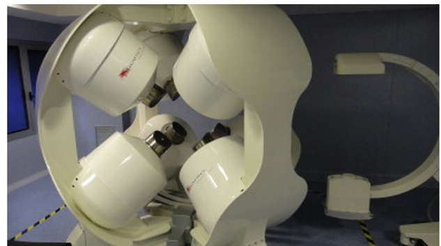
Fig. 5 The CGCI system incorporates eight electromagnets fixed in a spherical configuration. Reproduced with permission [81]. Copyright 2013, Elsevier
