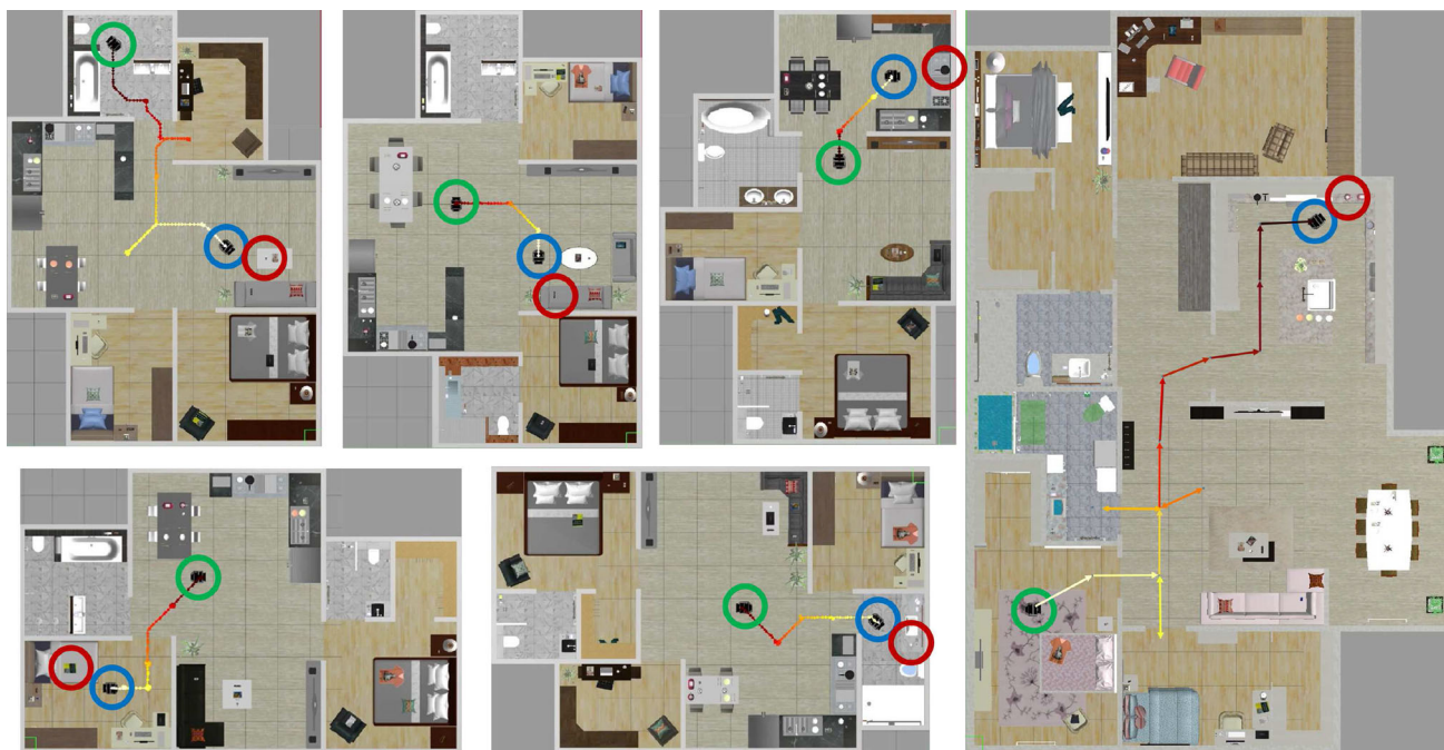
Fig. 5 Example search paths generated by the proposed approach from different object search trials. The green circles correspond to the robot's initial locations, and the blue circles correspond to its final locations. The red circles indicate the locations of target objects (color figure online)
