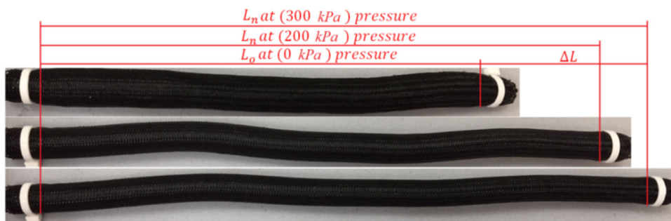
Fig. 2 The extensor muscle with different supplied pressures, where: L_o is the muscle length at the rest, L_n is the muscle length under pressurization and \Delta L is the amount of length increase
