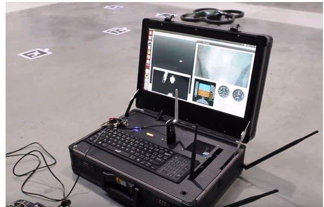
Fig. 2 Intel miniITX-based ground station for off-board processing and control
