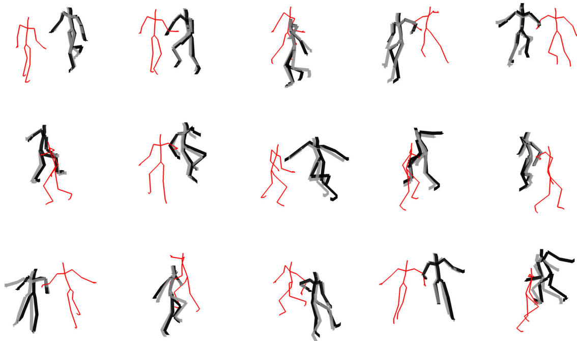
Fig. 6 Example of TP-MFA to encode and retrieve full-body dancing motion from [36]. Here, the motion of one of the two partners ( D = 94 ) is retrieved by adapting it online to the motion of the other partner. In the model, the red stick figure (in thin line) is the frame of reference and the gray stick figure (in thick line) is the motion encoded in TP-MFA. The black stick figure (in thick line) shows the motion regenerated with TP-MFA and Gaussian mixture regression, based on the observation of the
