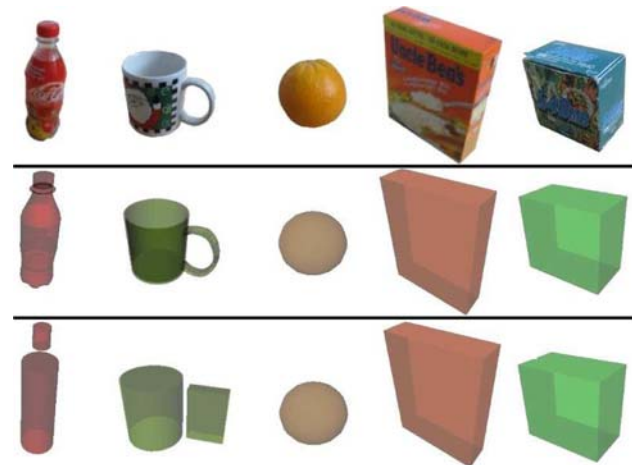
Fig. 4 Top the real objects. Middle the detailed object models. Bottom the simplified models, object primitives
