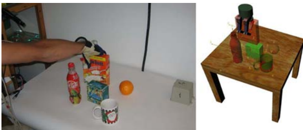
Fig. 5 Left the human moves the rice box. The system recognizes what object has been moved and which grasp is used. Right the robot grasps the same object using the mapped version of the recognized grasp
