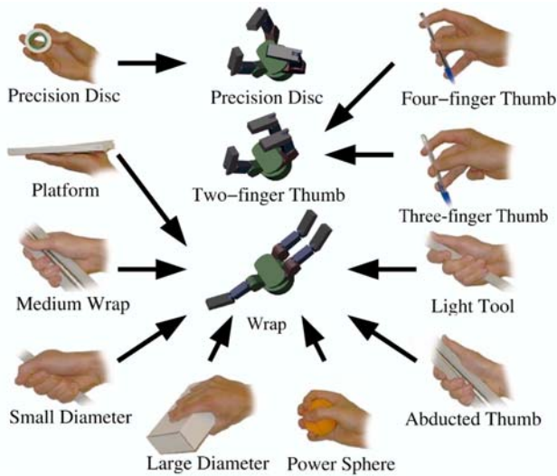
Fig. 1 Mapping a selection of grasps from Cutkosky’s grasp hierarchy to three Barrett grasps. The robot hand configurations shown are the initial joint positions
