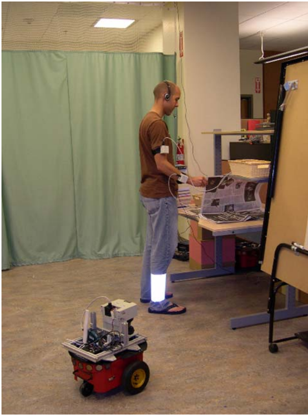
Fig. 5 The first experimental setup: the participant is performing Task 4 (turning pages of a newspaper) with the robot at a social distance. The laser fiducial is on the participant's right leg, the motion sensor on the right arm, and a microphone is worn on standard headphones
