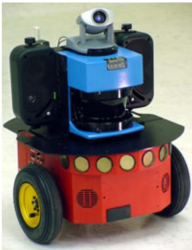
Fig. 4 Robot test-bed; an ActiveMedia Pioneer 2-DX mobile robot equipped with a SICK laser range scanner, a camera, and speakers
