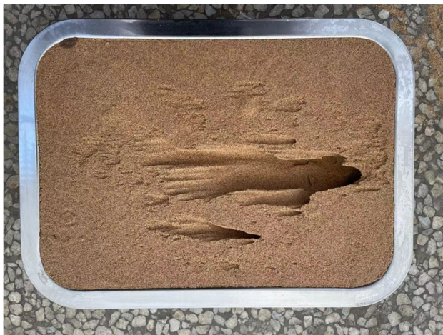
Fig. 7 The broken crust and the hollowing out of inner sand
