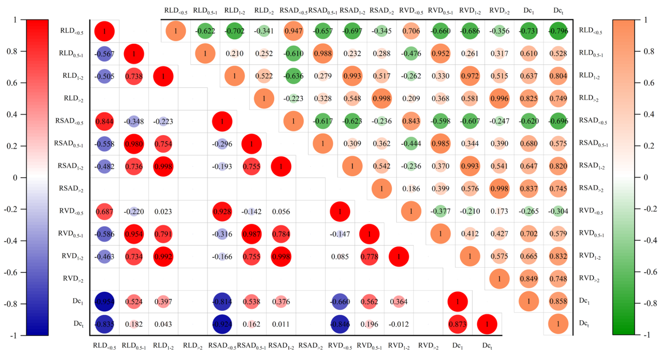
Fig. 8 Correlation results between the soil detachment capacity ( D_{c1} , D_{c2} ) and root parameters in different diameters. Among them, relevant results of fibrous roots is at the lower left of this picture, while taproots is at the top right of this picture
