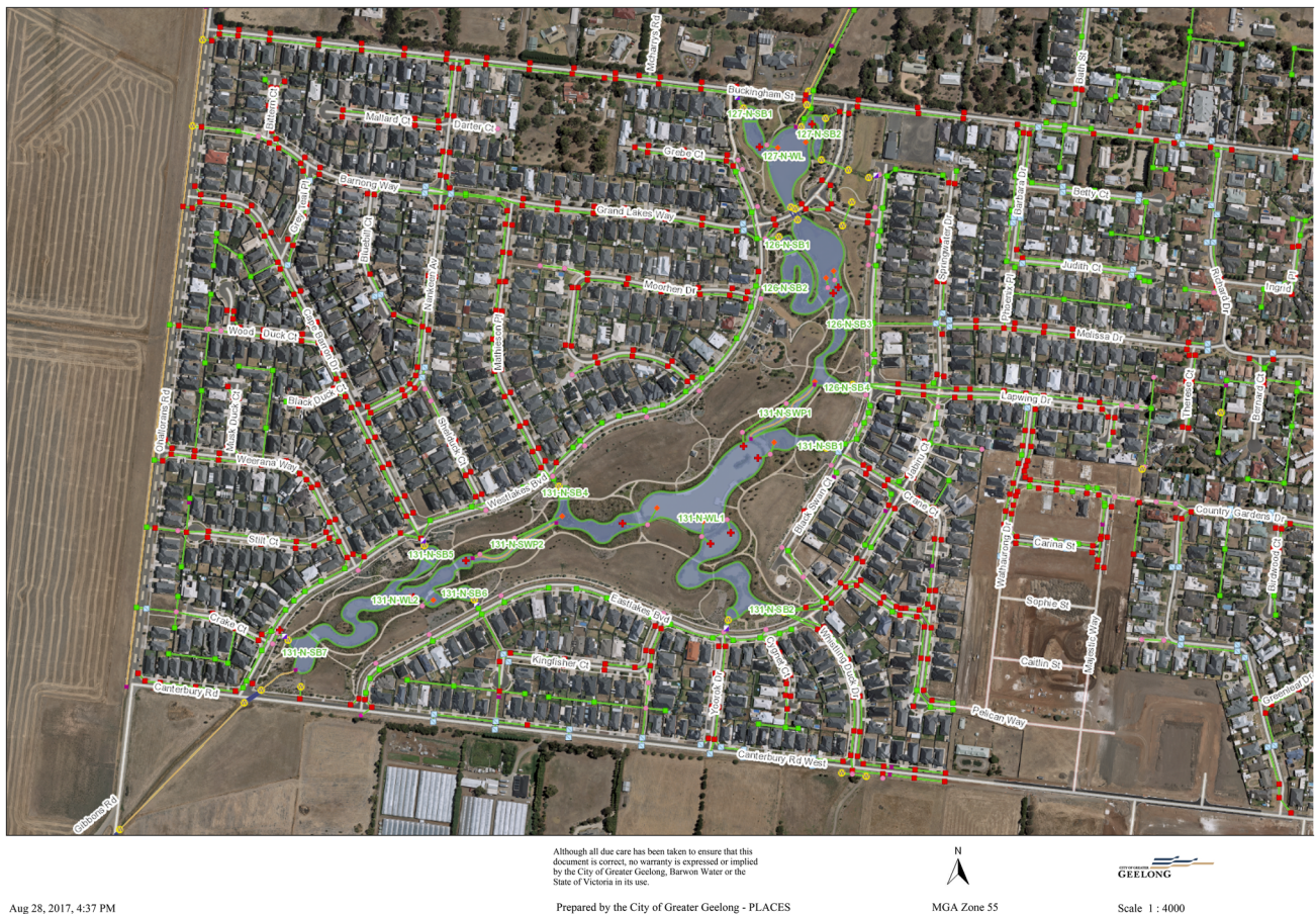
Fig. 3 Grand Lakes constructed wetland and NbS area. Green lines represent major subsurface drainage pipes, red dots represent catch-basin locations, and yellow lines represent surface drainage channels
