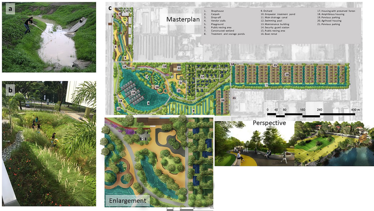
Fig. 1 Progression of stormwater design visions: a Simple stormwater pond, primarily for runoff quantity detention, Buffalo, NY, USA (photo by authors), 1970s–early 2000s; b bioretention cell (raingarden, Singapore) as an example of WSUD, 2010s–present, with substantial depth for surface storage and four substrate layers for additional storage and water quality treatment. Focus has been on individual features, as shown here, or distributed, small features; c NbS design (peri-urban Bangkok, Thailand), showing the Master Plan, including an integrated, holistic vision for community wellbeing and optimization
