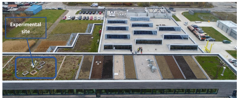
Fig. 1 Experimental site of four raised beds established on the green roof at the University Centre of Energy Efficient Buildings, Czech Technical University in Prague
