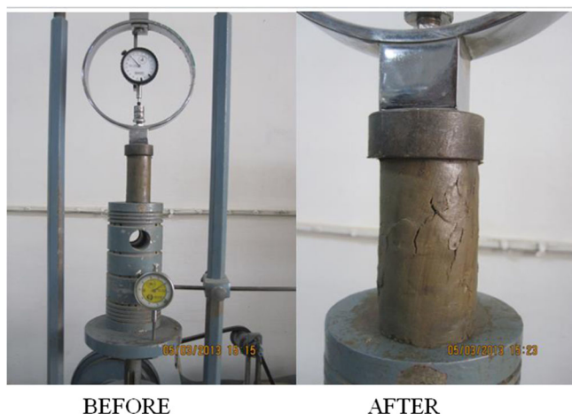
Fig. 3 Sample before and after the test in the unconfined compression test apparatus
