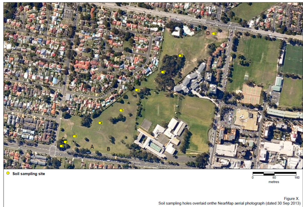
Fig. 1 Research area, AB —Hawkesbury Sandstone, CE —Wianamatta Shale, D —Mittagong Formation sampling 1 to 9, was the initial transect to determine the background heavy metal level
