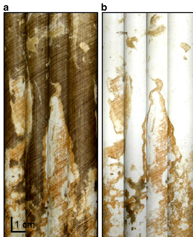
Fig. 3 Image of a Mn redox bar before (a) and after (b) protrusion into acidified hydroxylamine hydrochloride (AAH) solution for 10 min
