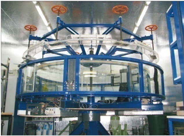
Fig. 1 Annular flume at the Institute for Hydraulic Engineering and Water Resources Management, Aachen, Germany (picture: C. Cofalla)
