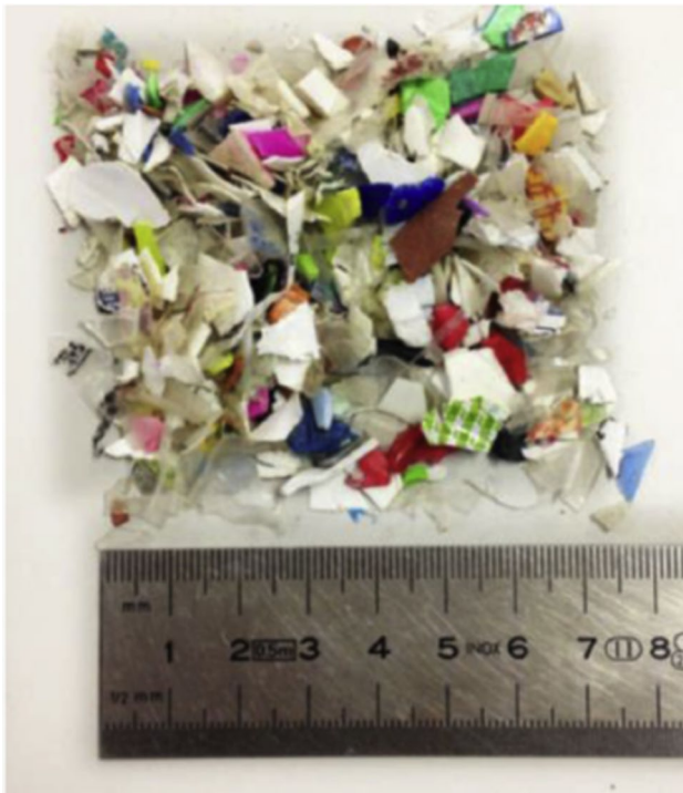
Fig. 5 Recycled mixed PP scales incorporated in model A vault (7.3) as raw material (Rubio-de Hita et al. 2018)
