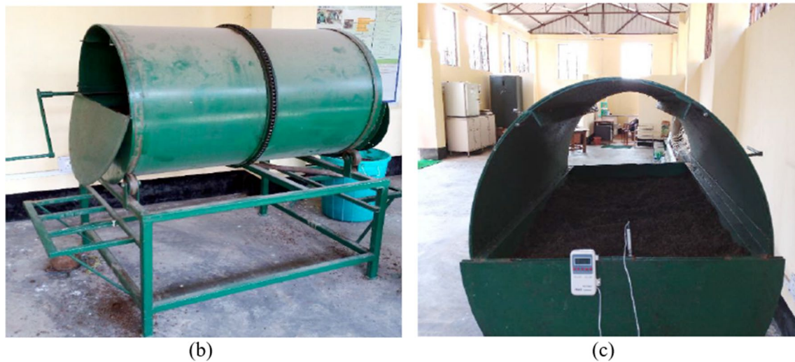
Fig. 3 Schematic diagram of rotary drum composter and b and c rotary drum composter
