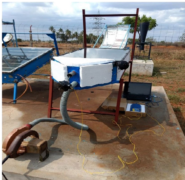
Fig. 2 DPSAH system installed at the energy park
