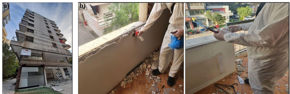
Fig. 4 One of the target buildings (a) and sampling from wall covering (b)
