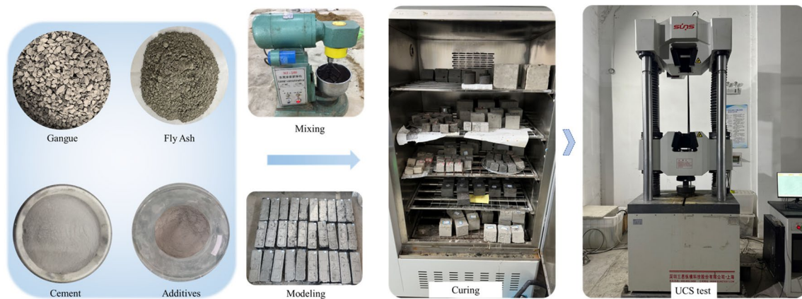
Fig. 2 GCBM’s mechanical testing process
