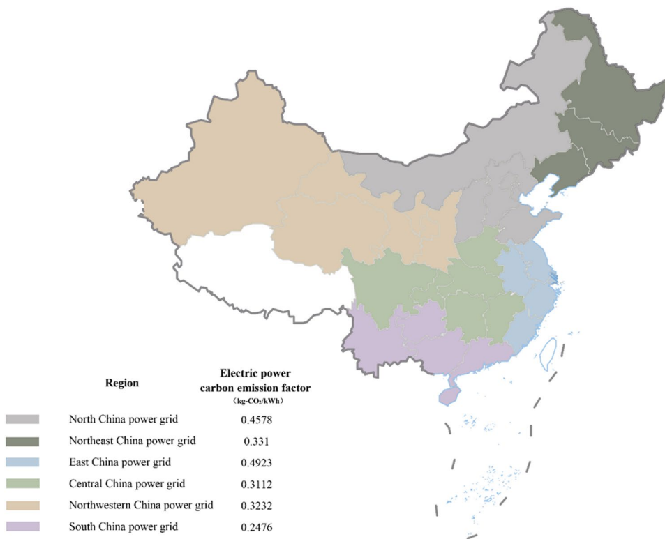
Fig. 1 Carbon emission factors of the regional power grid in China. (Data source: Carbon emission factors of China’s regional grid baseline for emission reduction projects from 2006 to 2017)
