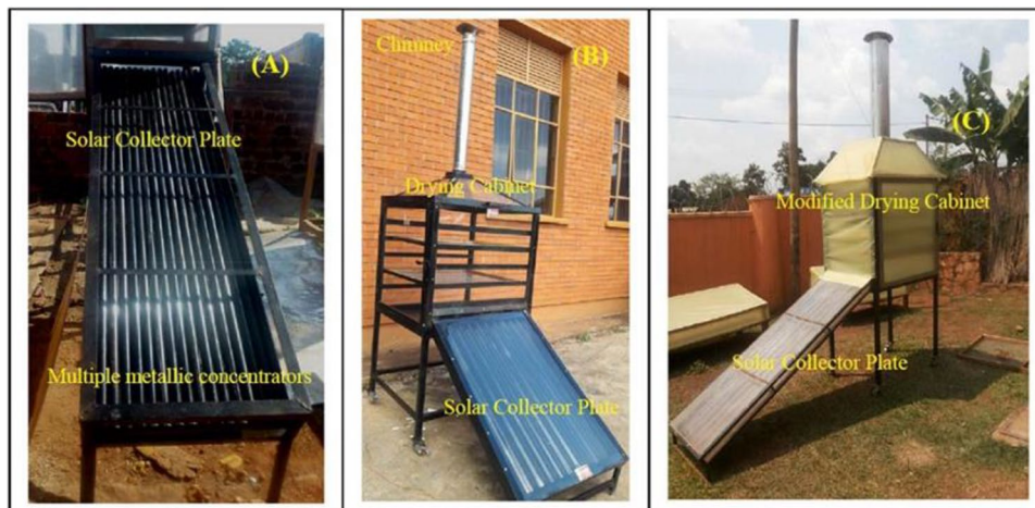
Fig. 7 Photos of an improved hybrid indirect passive (HIP) dryer: A a modified solar collector plate consisting of multiple metallic solar collectors; B , C the physical prototypes of the HIP without and without a non-perforated greenhouse plastic cover enclosing the dryer cabinet (Ssemwanga et al. 2020)
