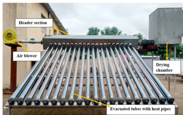
Fig. 12 Photographic view of evacuated heat pipe solar dryer (Mathew and Thangavel 2021)
