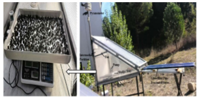
Fig. 10 Experimental setup of solar sludge dryer (Amin and Salihoğlu 2021)
