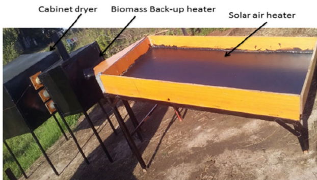
Fig. 20 Solar air heater assisted by biomass back-up heater (Chekol et al. 2021)
