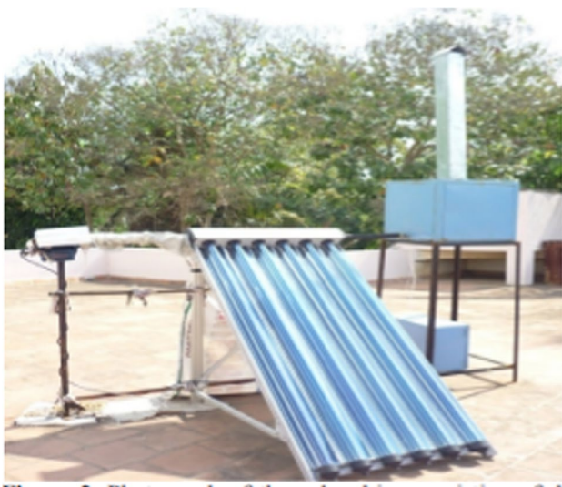
Fig. 11 Photograph of evacuated tube collector-based solar dryer (Umayal Sundari et al. 2014)
