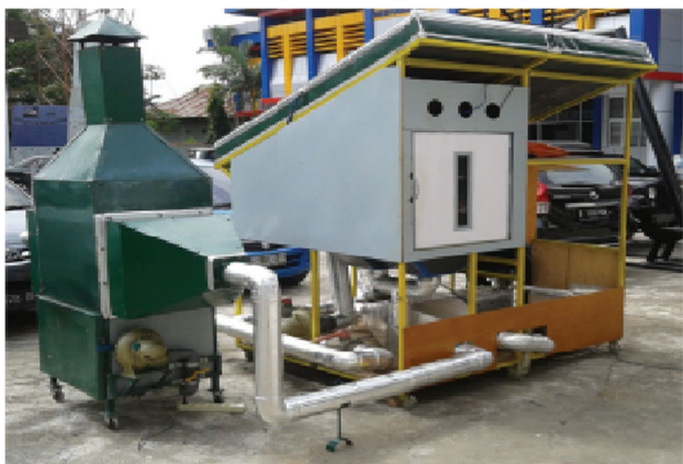
Fig. 21 Photograph of the solar-assisted heat pump drying integrated with biomass furnace (Yahya 2016)
