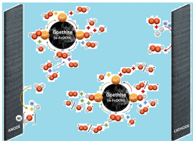
Fig. 4. Electro-Fenton reaction mechanistic scheme using goethite particles as heterogeneous catalyst. Adapted from Poza-Nogueiras et al. (2018)
