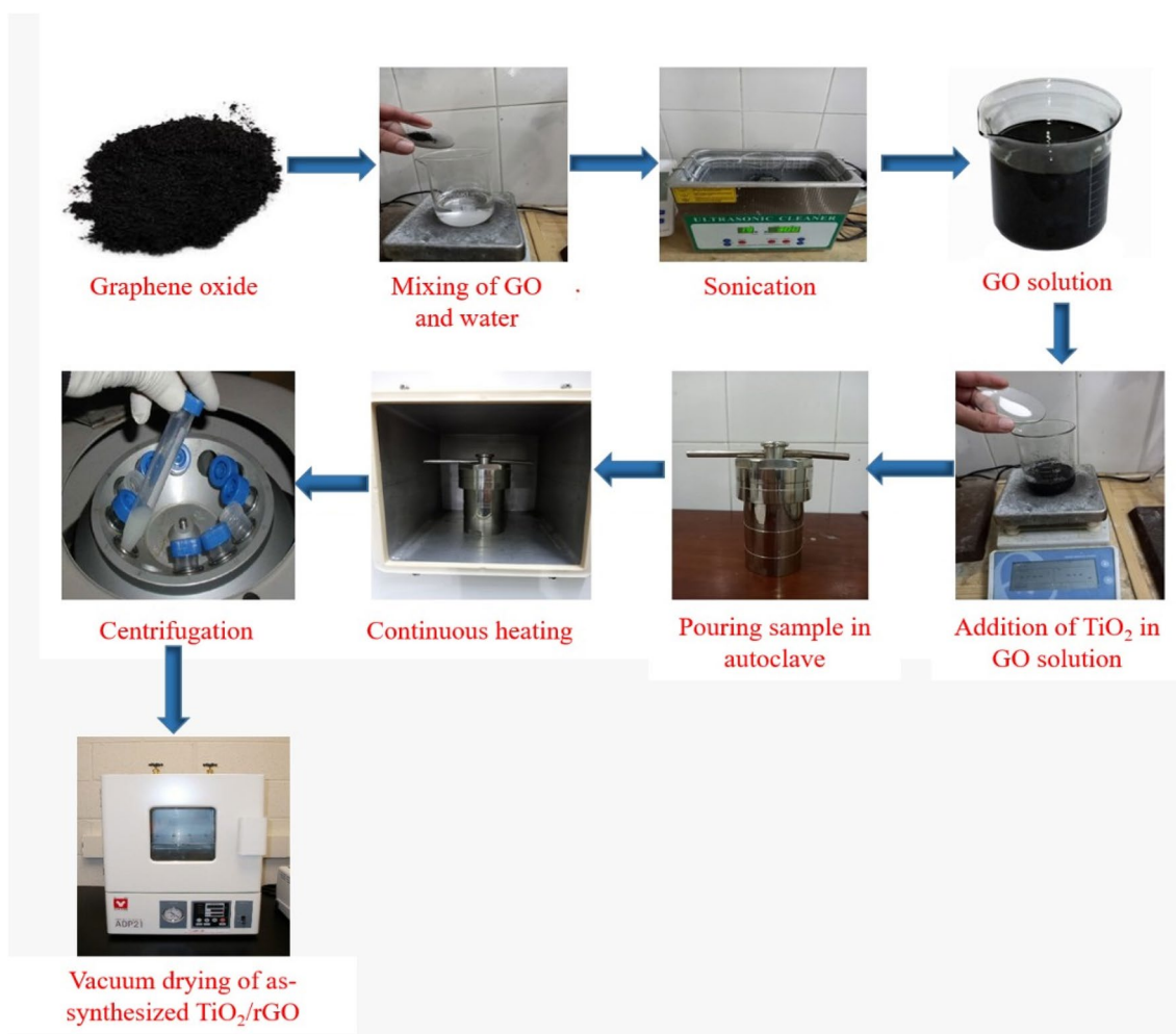
Fig. 1 Experimental procedure for step-wise synthesis of TiO 2 /rGO
