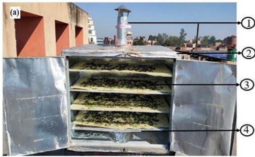
1. Chimney 2. Drying chamber 3. Tulsi leaves 4. Trays
