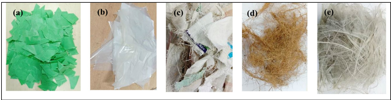
Fig. 2 Images of the raw materials a HDPE, b , LDPE, c PP, d coconut fiber and e jute fiber
