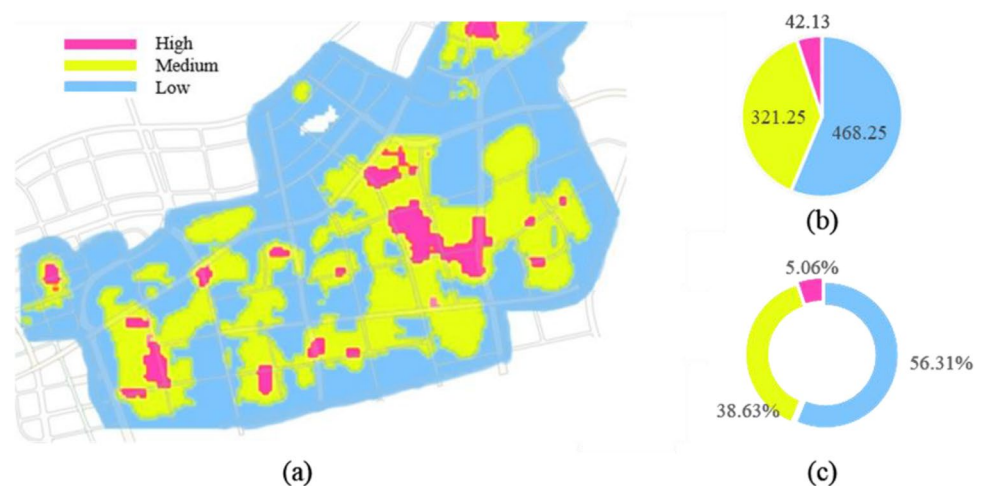
Fig. 6 Comprehensive assessment of urban flooding risk in the study area: a the distribution of each risk level, b the occupied area of according risk level ( \text{hm}^2 ), and c proportion of areas with corresponding risk level
