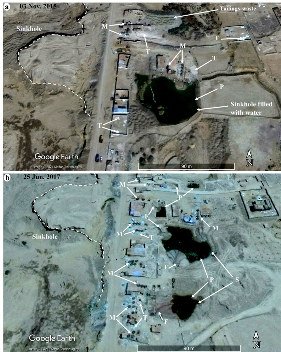
Fig. 7 Temporal Google Earth high-resolution multispectral images showing the distribution, setting, development (2015–2017), and potential environmental impact of a gold processing site over the karstic plateau in El-Idwa village, southwest of Wadi Abbadi outlet, where depressions (outlined by white dashed lines) are being utilized as amalgamation ponds (P; dark polygons). Also shown is the distribution of associated wet-pan mills (M) and gold tailing heaps (T). Note the increase in gold processing activities between November 2015 and June 2017, as evidenced by the rise in the number of mills (M) and the fan-shaped drainage patterns (F) emanating from each of the ponds and flowing towards, and draining in, sinkholes (S) where the Hg-rich waste is disposed. A red box in Fig. 2c outlines the location of Fig. 7
