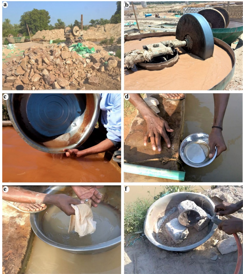
Fig. 3 Field photographs show Au-Hg amalgamation and gold extraction processes associated with ASGM activities in the study area. a) Crushing ore rocks from small-scale and abandoned gold mines in the Eastern Desert. b) Milling crushed ore with elemental mercury in a wet pan to create a slurry. c) Washing out the slurry to separate the amalgamated residue. d) Hand-picking of the Au-Hg amalgam. e) Refining the amalgam by squeezing out excessive mercury using a cloth. f) Burning the amalgam to vaporize the mercury and produce gold sponge particles
