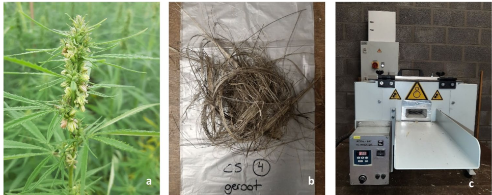
Fig. 6 a Hemp at 50% flowering; b hemp fibers from field retted hemp; c lab-scale decorticator (breaker)
