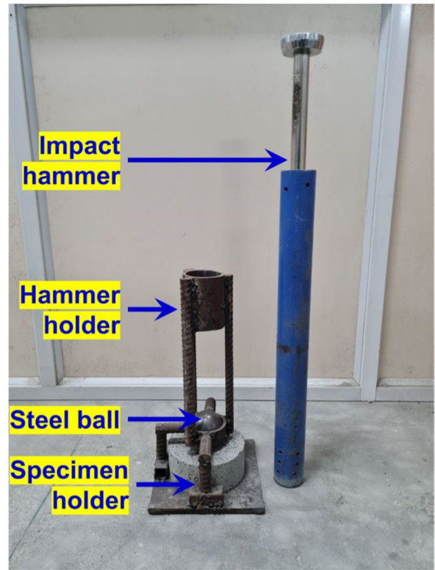
Fig. 2 Drop weight impact test setup
