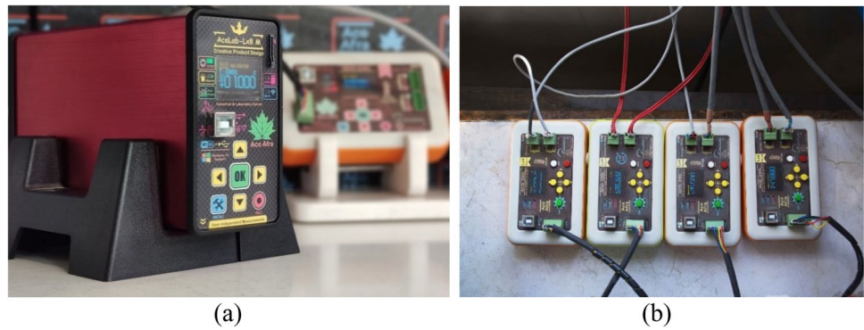
Fig. 4 (a) AcoLab-Lx8 Data logger server, and (b) Different temperatures and current data logger modules for measuring CPC collector variables
