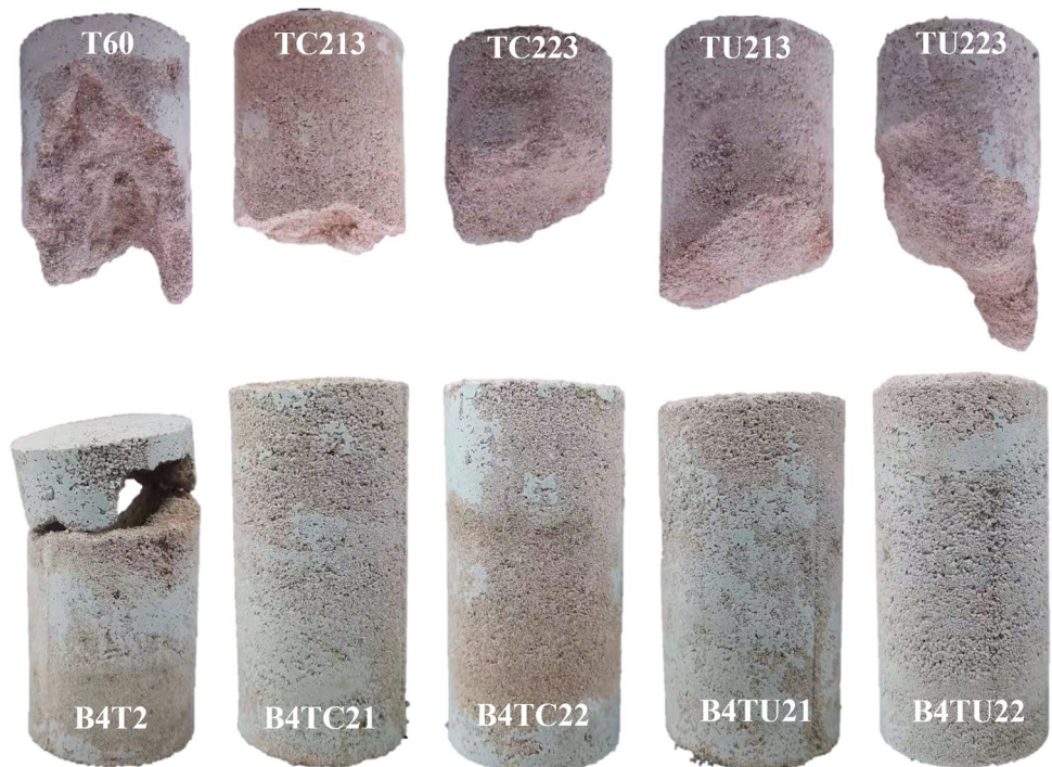
Fig. 4 Physiognomy of microbially cured Pisha sandstone
