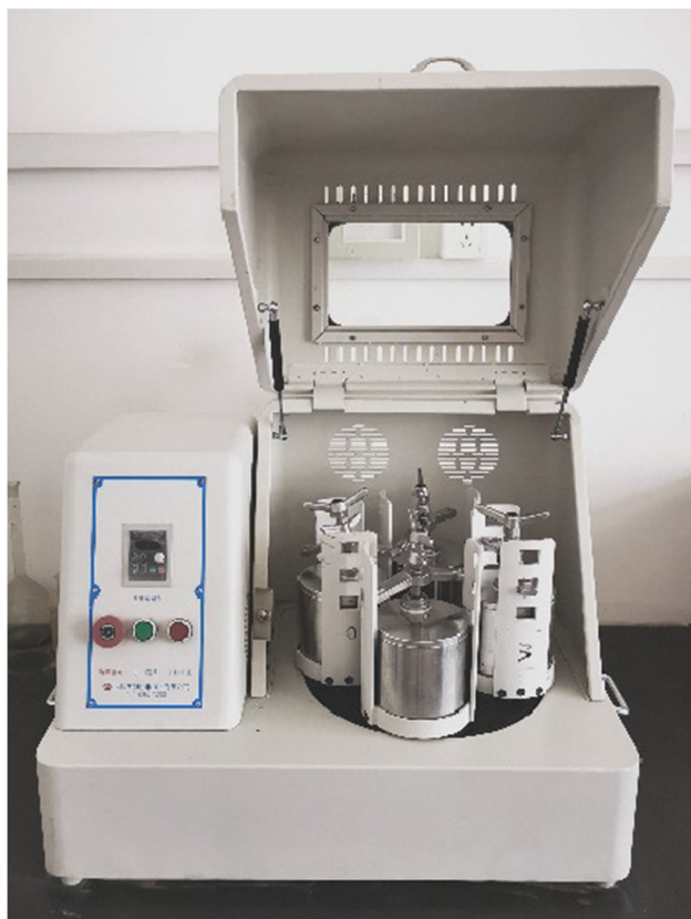
Fig. 4 Internal structure of the planetary ball mill
