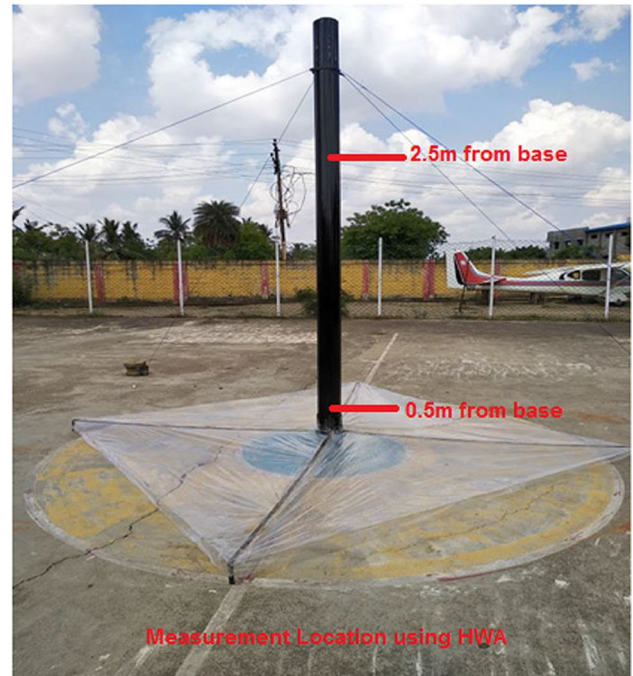
Fig. 3 Experimental setup of exp. 1
