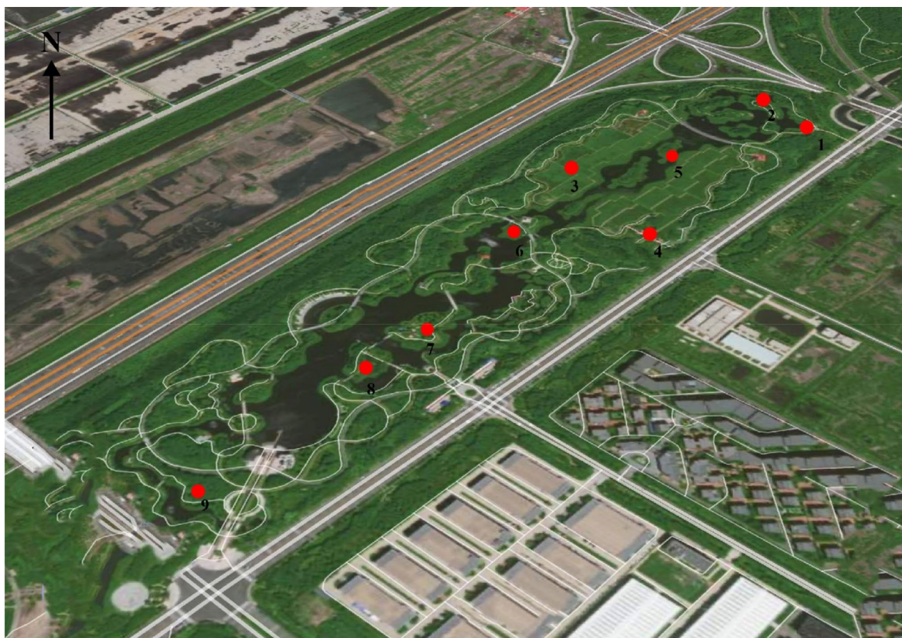
Fig. 1 CW sampling point layout. 1 From water inlet; 2 from regulation pond; 3–4 from subsurface flow wetland (SSF CW); 5 from surface flow wetland (SF CW); 6–8 from landscape lake; 9 water outlet
