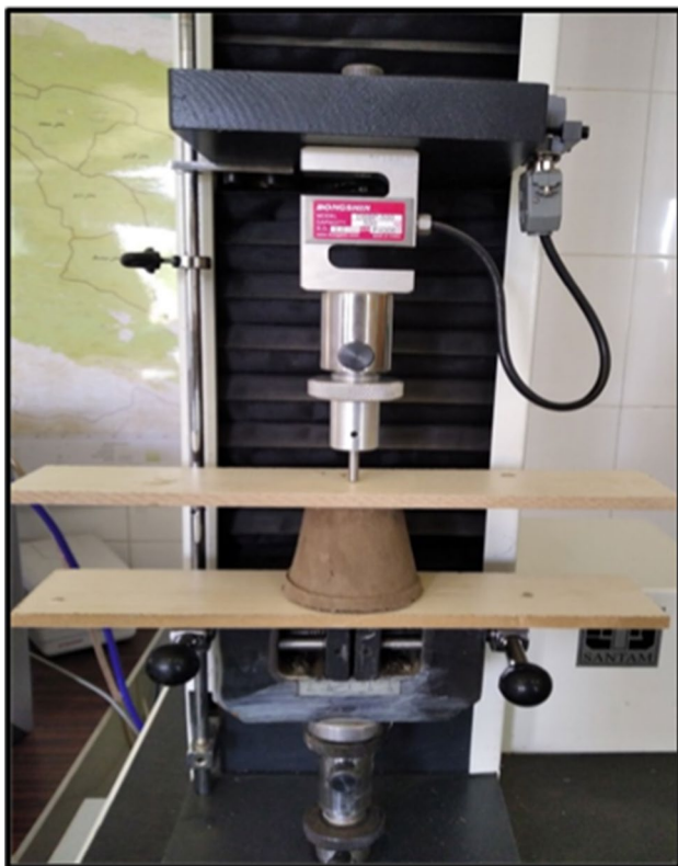
Fig. 6 Internal bonding. Sample placement within the test frame
