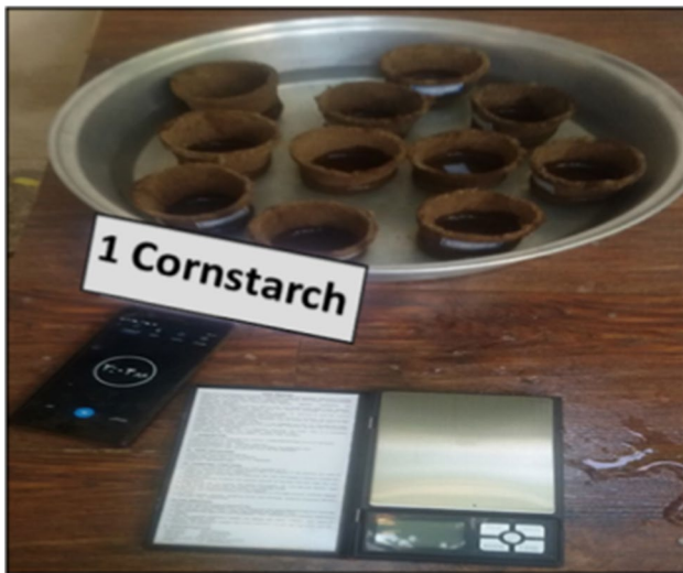
Fig. 4 Water absorption (WA) test assembly. An iron pot, a cell phone timer, and a laboratory scale were used to record WA at 15-min intervals for each sample pot
