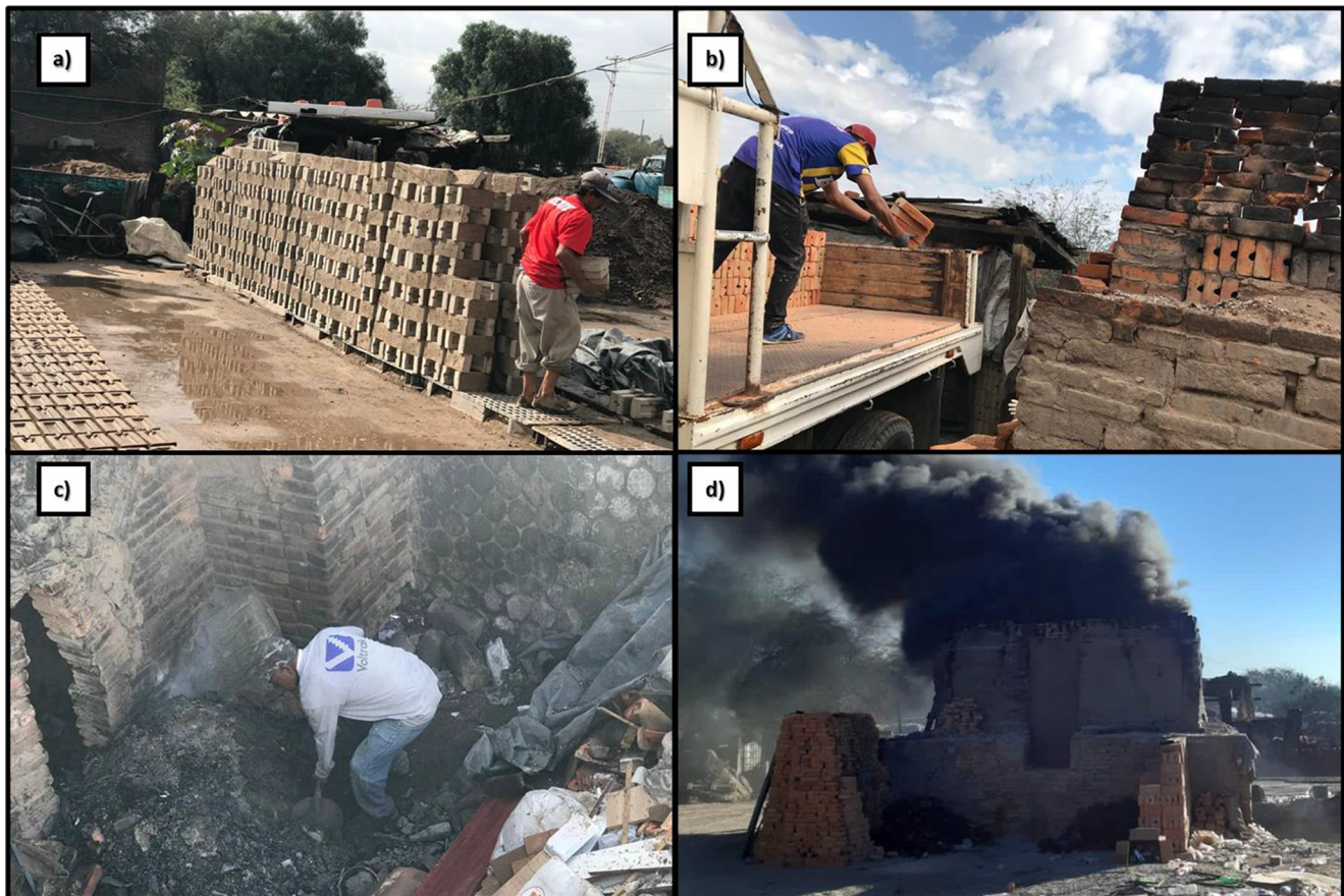
Fig. 1 Stages of the brick making process in San Luis Potosí, “Las Terceras”. a Molding, b brick arrangement in the oven, c fuels, and d burning the brick in the kiln
