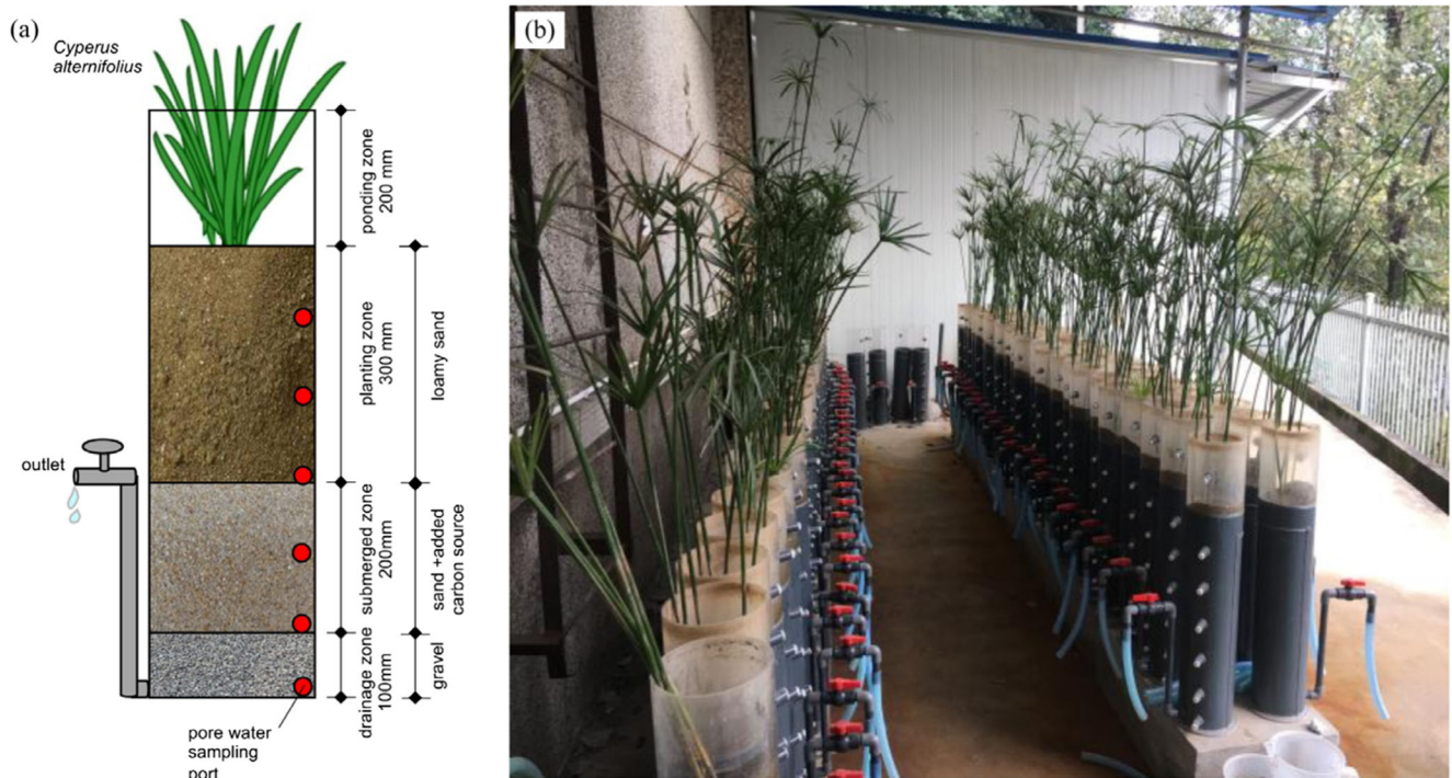
Fig. 1 a Schematic diagram of the biofilter columns and b experimental set-up of bioretention consisting of 126 columns
