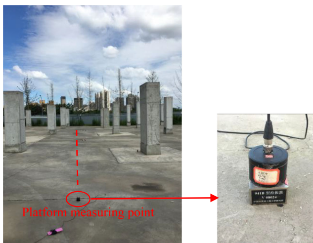
Fig. 9 Sensor setups on the platform
