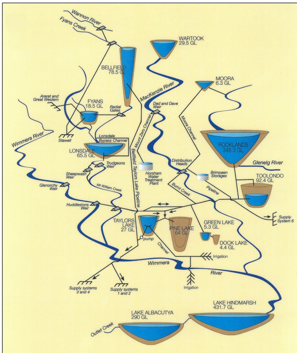
Fig. 2 Schematic diagram of the complex water supply in the Wimmera-Glenelg system (Courtesy of GWMWater)
